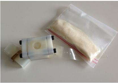
Fig. E4. Skin model: gelatin powder, polyurethane membrane, and skin model mount.
