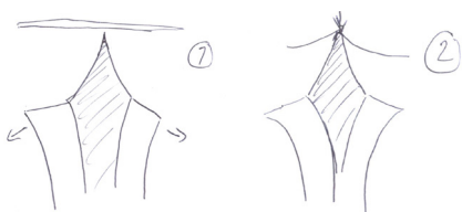
Fig. D7. 1) the elastic material bents 2) The needle tip is compressed.
