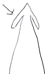
Fig. D1. Needle tip deforms it self sharp.
