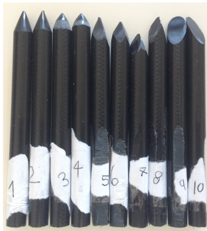
Fig. E2. POM needle with different tip geometries
