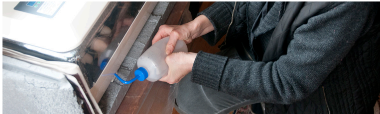
Adding water for humidity
