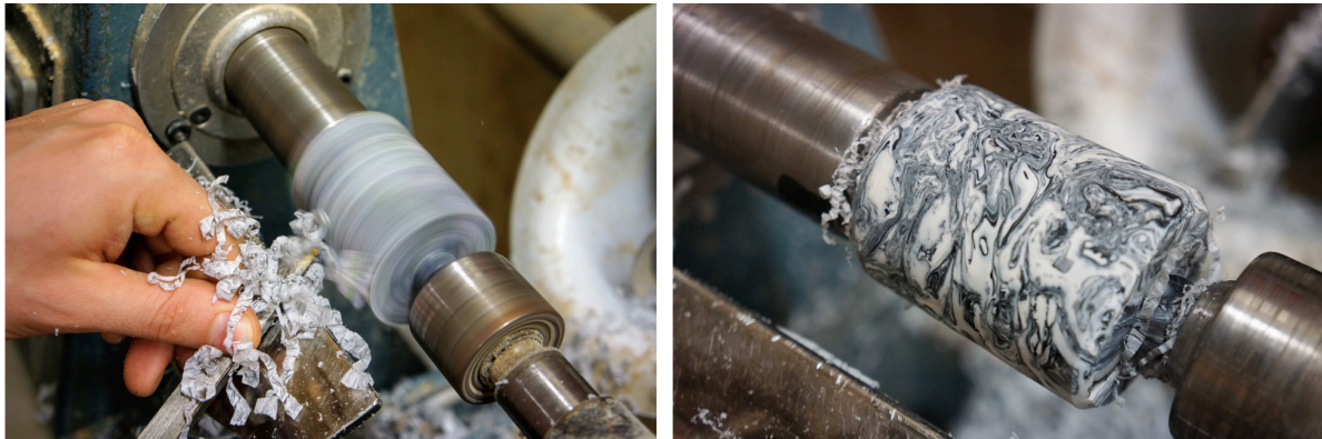
Figure 8.12 Post-processing a block of PE on the lathe yields new textures (Prototype 2.1)
