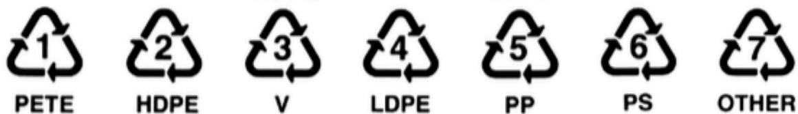
Figure 4.1 The SPI Plastic packaging identification system. American use V for the Vinyl in PVC (Christensen 2011)
