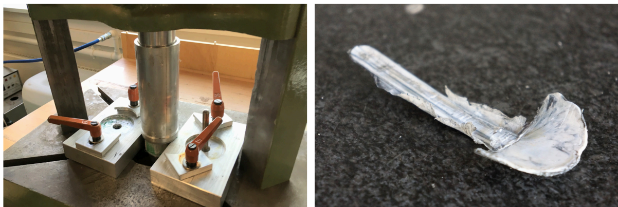
Figure 8.9 The part and core is pressed out of the mold (left) A runner showing the effect of the overflow groove (right)
