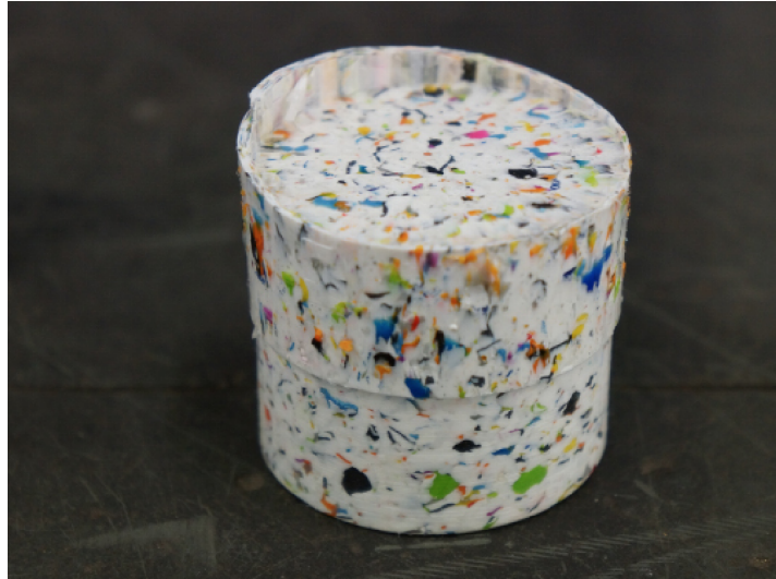
Figure 8.13 Cylindrical part made from shredded plastic
