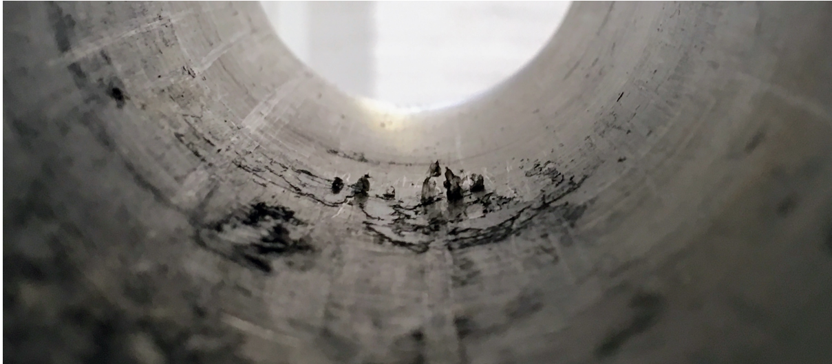
Figure 8.11 Plastic film and blobs sticking to the inside of the tube
